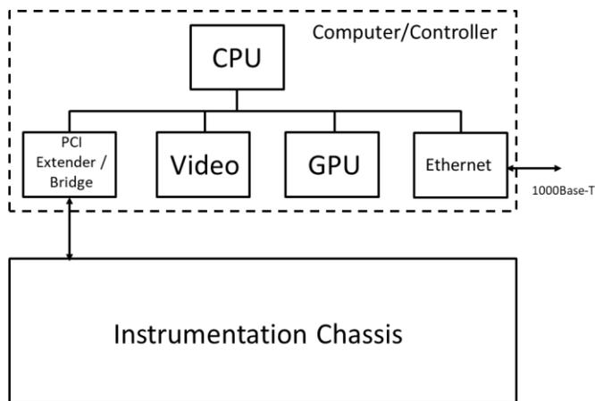
Figure 1 – PCI extends the computers PCI bus to an external instrument chassis that houses instrumentation cards.
