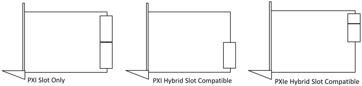
Figure 3 – A comparison of PXI and PXIe cards and their backplane connectors.
